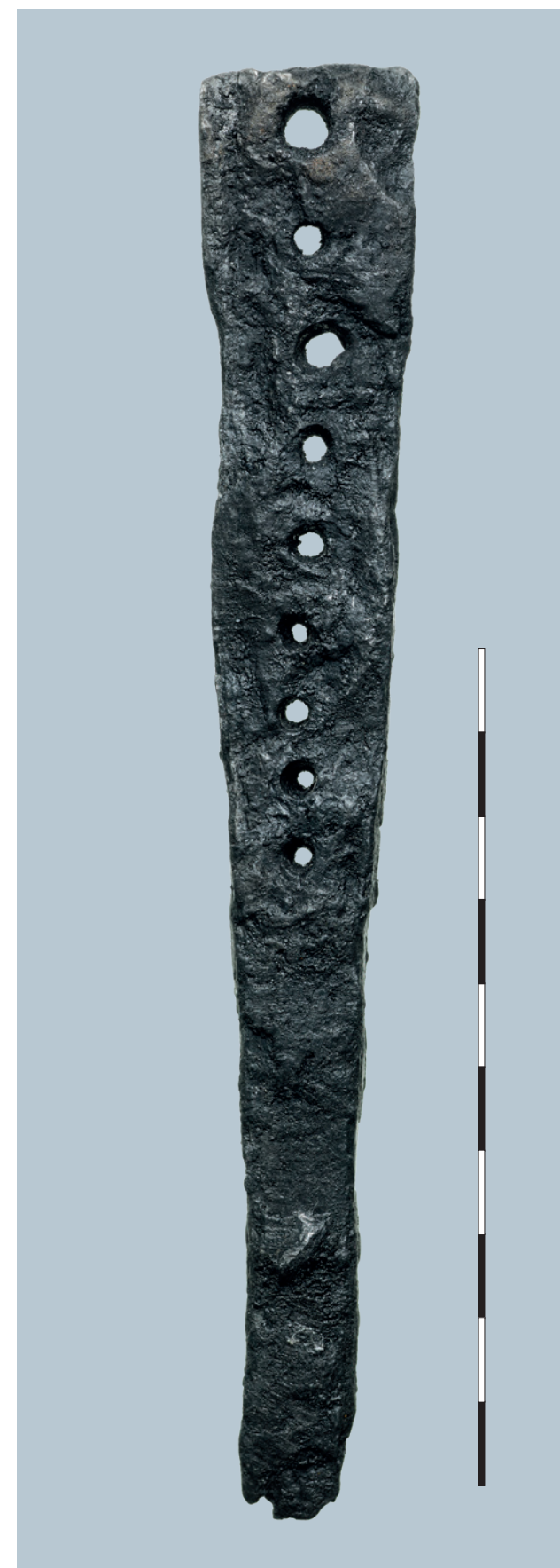
Figure 17. Drawplate used in the production of iron wire. Metal-detector find from Mysselhøjgård.
